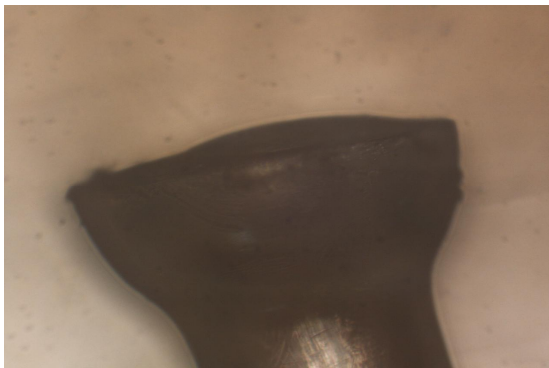
Fig. 6. Lens tip POF with Unpolished edges
